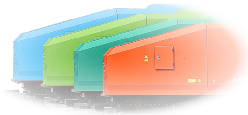
Diesel, mild hybrid, electric and range extender series are developed on the same platform, with 85% of structural parts common.
